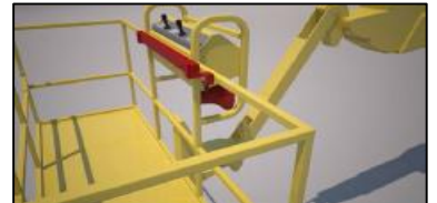
Pressure sensing device – bar when activated ceases further movement and activates alarm
