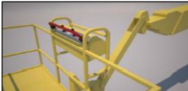
Pressure sensing device – breakaway bar when activated ceases further movement and activates alarm
