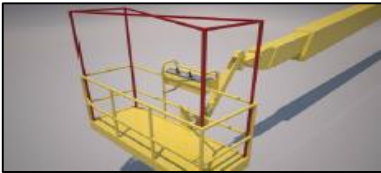
Physical barrier – Fixed full cage structure
