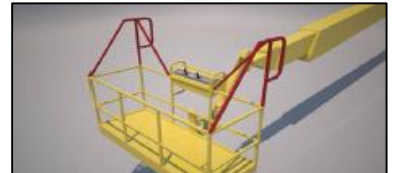
Physical barrier – Side protection barriers
