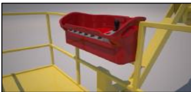
Pressure sensing device – when activated ceases further movement and activates alarm
