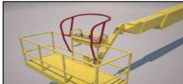
Physical barrier – Operator protective structure
